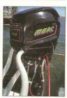
Brackets and such were bolted through the gorgeous, flow-coated, balsa wood flooring; anodized purple hardware and purple gelcoat established the clean tone of the installation. Wiring was neatly routed and loomed, in line with top industry standards.
