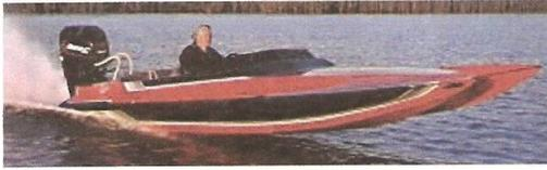
The 300 Pro-Max is a big outboard. So big, it dwarfs the others when parked next to them, even though it's still just a V-6. At 183 cubic inches, it's 30 cubes larger than the 225 and 2.5. The massive powerhead is supported by an even beefier center section, which is custom built for the 300 alone. The Merc factory provides open exhaust as standard equipment, but the 300 isn't as loud as the 2.5
